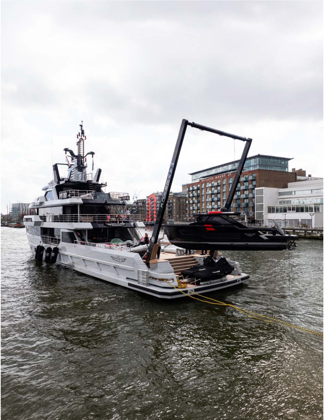
TENDER LAUNCH WITH THE A-FRAME
