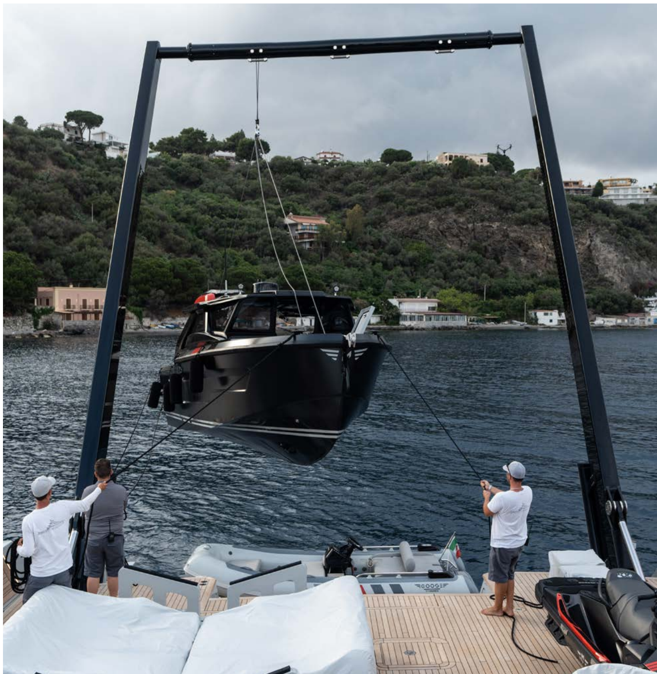
TENDER LAUNCH WITH THE A-FRAME
