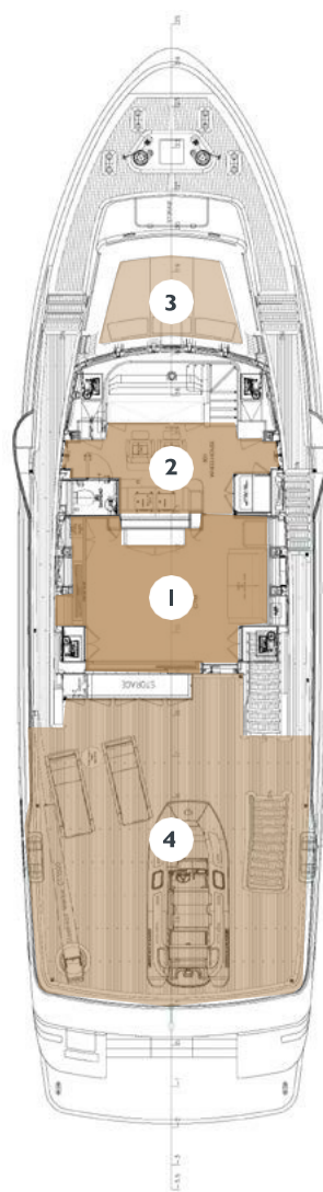
1. SKY LOUNGE 14,6 sqm / 157.1 ft 2 2. WHEELHOUSE 8.2 sqm / 88,2 ft 2 3. SUN BED 5.7 sqm / 61,3 ft 2 4. OUTDOOR AREA 46.8 sqm / 503.9 ft 2
